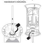
Return shroud to unright position after finishing operation. Leave tubing attached to tube-fed safety syringe and quick-fit connector until dosing equipment has been removed from the shroud. Remove dosing equipment by pushing the trigger as shown in the picture, then disconnecting the quick-fit connector
