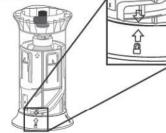
the fluid connection, Attach the quick-fit connector to tubing if not already attached. Push the quick-fit connector downwards onto the shroud fitting until it clicks into place.
